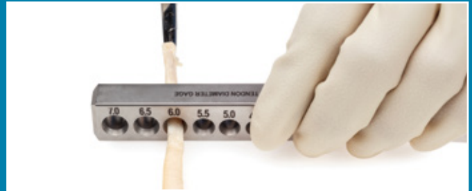
Figure 4. The tendon is fitted through the gauge opening for the diameter measurement.
